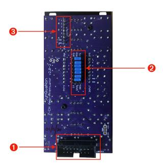
1 A100 Bus Keyed power connection with reverse polarity protection. Red stripe is on the left.
